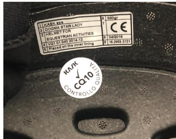
*This helmet standard was located underneath the liner – this is a VG1 helmet standard.*
